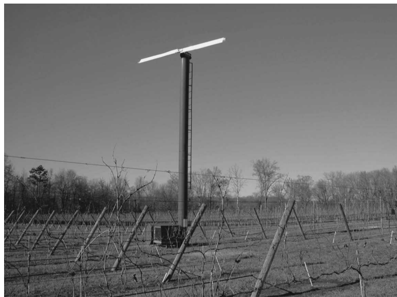
Fig. 5. This Orchard-Rite, Ltd. (Yakima, WA) wind machine stands 10.7 m above the vineyard floor and has a gas-powered engine that turns a 5.8-m fan. It protects a 2.83-ha vineyard in Davidson County, NC. The fans or propellers minimize cold air stratification in the vineyard and bring in warmer air from the thermal inversion. The amount of protection or temperature increase in the orchard depends on several factors. However, as a general rule, the maximum that the air temperature can be increased is \approx 50\% of the temperature difference (thermal inversion strength) between the 1.8- and 15.2-m levels. Thus, these machines are generally not very effective with minimum temperatures below -2.2^\circ\text{C} . (Photo by Barclay Poling, 18 Dec. 2005.)
